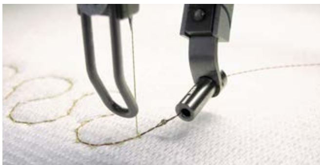
Insertion of a conductive thread into a textile layer (source: STFI)
